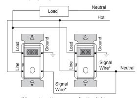
When using a three-way application, lights may be turned on from either switch, but can only be turned off at the switch that turned them on.
