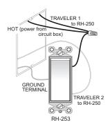
The RH-253 may be used with the RH-250, as shown in these drawings, or with a CH-250, CD-250, CU-250 or RD-250 multi-way sensor in place of the RH-250.
