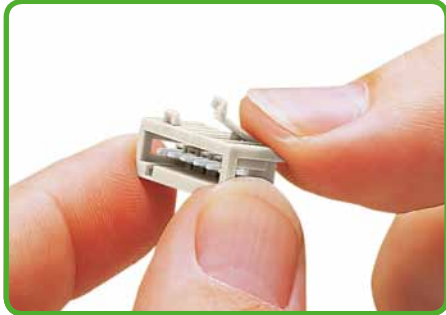
Coding a male header - fitting coding key(s).
