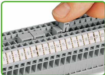
Commoning with adjacent jumpers. Push jumper down until fully inserted!
