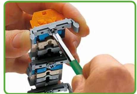
Terminal strip with fixing flanges, screw mounting of 209-123 mounting adapter (distance between mounting adapters should be 35-40 mm).
