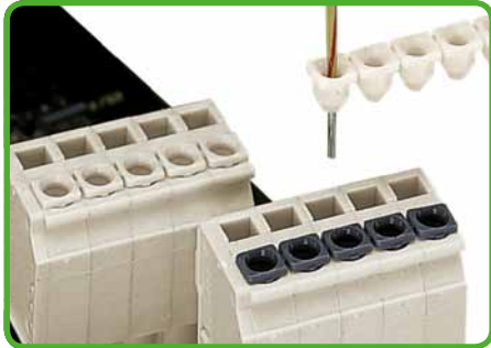
The insulation stop prevents the insulation of smaller conductors from being inserted into the clamping unit.
