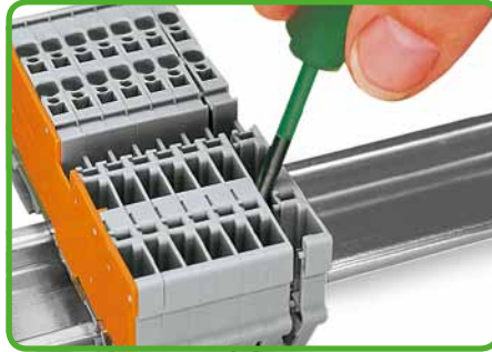
Unlock assembly with (3.5 x 0.5) mm screwdriver and remove terminal block via release lever.
