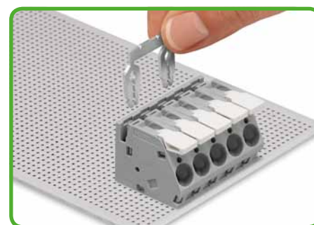
Commoning via comb-style jumper bar.
