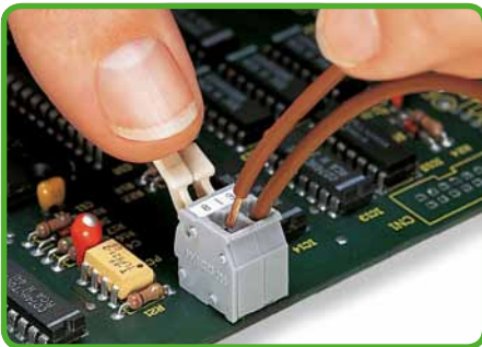
Inserting/removing conductor via finger-operated lever - 255 Series.
