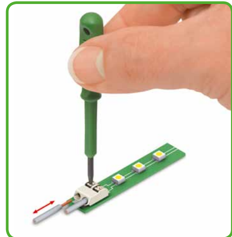
Inserting/removing fine-stranded conductors by lightly pressing on push-button (e.g., using a 233-335 operating pen).
