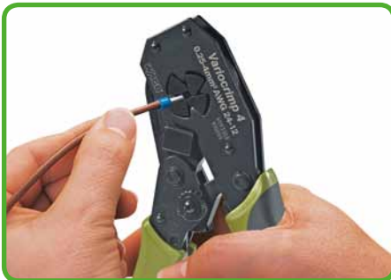
Introduce ferruled conductor into crimping station. Squeeze handles until ratchet mechanism is released.
