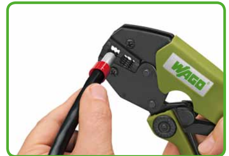
Insert ferruled conductor into crimping station.
