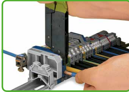
The plunger is placed into the upper operating slot of the side-entry terminal block and the clamp is hooked into the lateral operating slot. The contact is fully opened by pressing the handles together until they engage. Insert stripped conductor until it hits backstop.
