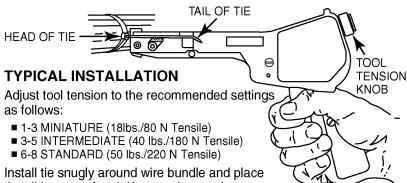
Install tie snugly around wire bundle and place tie tail in nose of tool. Keep tool nose close to head of tie. Squeeze tool handle (repeat if necessary) until tail of tie is cut-off. On return stroke, turn tool sideways to eject tail.
