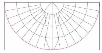
LED single board with internal reflector installed
