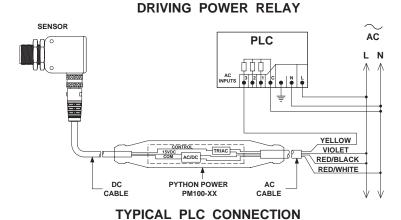
WARNING: Applied AC load must limit Python's TRIAC switch to rated current.
