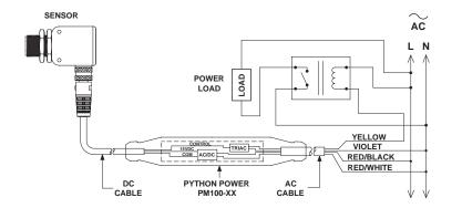
WARNING: Applied AC load must limit Python's TRIAC switch to rated current.
