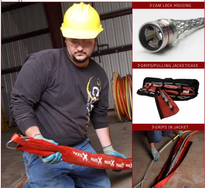
Fail-safe gripping system using both a cam housing and a double braided grip to quickly secure cable to rope without the fear of losing a conductor
