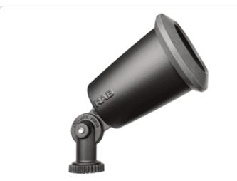
The economical R90 floodlight with a molded silicone external gasket to insure superior weatherproof seal. Polyester powder coating. PAR38 150 Watt max. Lamp not supplied.
