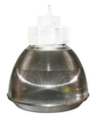
Indoor fixtures for use below 25'. 16" units for 250w Metal Halide. 22" units for 400w Metal Halide. Die cast aluminum housing and wiring box. Clear acrylic Lexalite Reflexor prismatic refractor. Ballast and lamp supplied.
