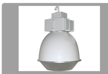
Indoor fixtures for use below 25'. 16" units for 250w Metal Halide. 22" units for 400w Metal Halide. Die cast aluminum housing, wiring box and semi specular anodized aluminum refractor. Ballast and lamp supplied.
