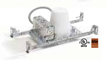
NS-401QAT 50W R/PAR20 4" Non-IC Airtight Line Voltage Housing Dia: 4-3/8" Depth: 5-3/4"
