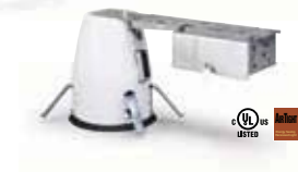
NSR-404QAT/10 50W MR16 GU10 lamp included 4" Non-IC Airtight MR16 GU10 Line Voltage Remodel Dia: 4-3/8" Depth: 5-5/8"
