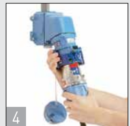
4 To reconnect, insert plug and twist. Pushing the plug fully home safely makes the circuit. The plug is held in the 'on' position by a locking ring. IP67 protection is enabled by fully rotating the locking ring in the clockwise direction.
