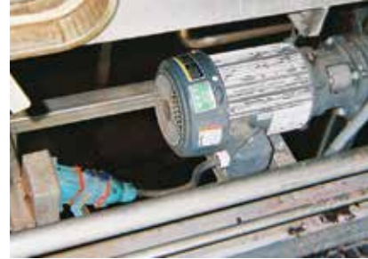
Decontactor™ plugs and receptacles are UL and CSA switch-rated up to 60 hp and 200A.
