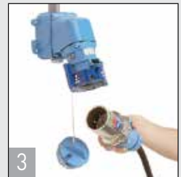
3 From the rest position the 'dead' plug can be withdrawn by rotating it counterclockwise. The receptacle can be made watertight up to IP67 by replacing the lid and turning the locking ring fully clockwise.
