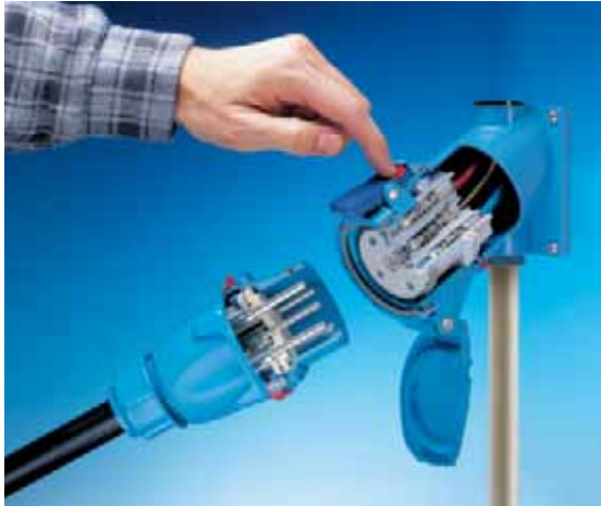
Pressing the pawl/button on the receptacle will safely switch off the DECONTACTOR. The plug can then be withdrawn in complete safety. (Cutaway model shown for illustration purposes)
