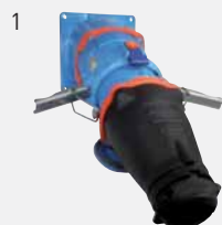
The plug is partially inserted, clamps are placed around tab, ready to pull the plug into the receptacle.
