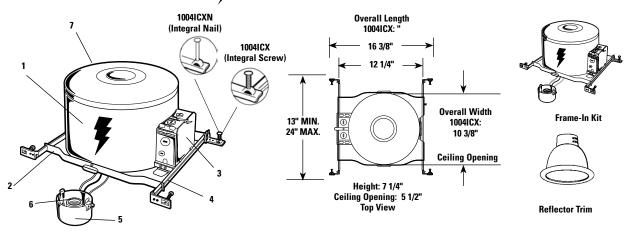
5" Aperture: Complete Fixture consists of Reflector Trim & Frame-In Kit. Select each separately.
