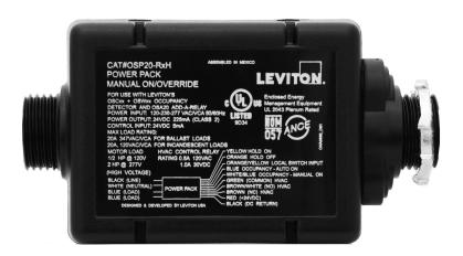
Containing both a 24VDC supply and a 20A line voltage relay for most models of occupancy sensors, the Leviton Compact Power Pack provides low voltage power and line voltage control for Leviton occupancy sensors. Versions include Auto-ON and Manual-ON inputs for occupancy sensors, Hold-ON and Hold-OFF capabilities and a local input for momentary or maintained dry contact switches.
