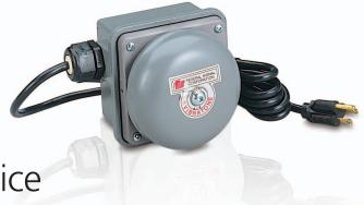
Federal Signal's TELB TelCom<sup>®</sup> Extension Ringer Device is a vibrating bell which is activated by the ringing signal of a telephone system. The TELB is specifically designed for use with an analog telephone. The ringing signal of 40-150VAC, 16-60Hz and local 120VAC power is all that is required to activate a TelCom signal.
