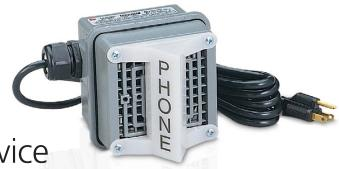
Federal Signal's Model TELC Extension Ringer Device is a horn and strobe combination signal which is activated by the ringing signal of a telephone system. The TELC is specifically designed for use with an analog telephone. The ringing signal of 40-150VAC, 16-60Hz and local 120VAC power is all that is required to activate a TelCom signal.
