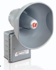
The Federal Signal Model AM15 is a rugged, re-entrant speaker for use in public address or paging applications. This 15 watt speaker features a rugged speaker cone and projector constructed of spun aluminum. The speaker wiring connections are enclosed in a dust- and moisture-proof, die-cast aluminum compartment. All external surfaces are sealed with gray powder coat paint.
