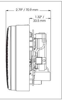
Operating Temperature: -65°F to 150°F -54°C to 66°C Non-metallic Polycarbonate Light Gray (RAL 7035) Housing: Net Weight: 1.0 lbs 0.45 kg Shipping Weight: 1.3 lbs 0.59 kg Height: 4.11" 104.4 mm Width: 4.11" 104.4 mm Depth: 2.79" 70.9 mm
