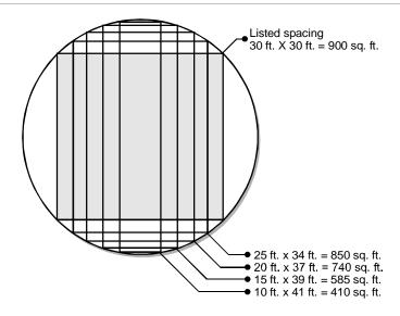
When installed on the ceiling, spot type heat detectors must be located a minimum of 4 in. (10 cm) from side walls. When installed on side walls, the detector must be between 4 in. (10 cm) and 12 in. (30 cm) from the ceiling, as shown below.
